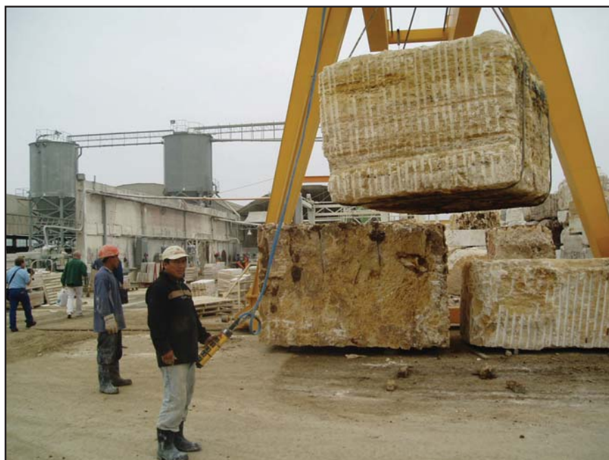
Waipouli Stone: Workers at a stone factory in Peru hoist massive blocks of Travertine stone quarried from the Andes. The high-quality, low-maintenance stone will be used at the Waipouli Beach Resort for things like kitchens, bathrooms, lanais and common areas.
